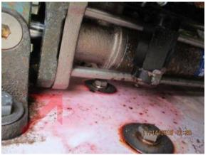
**Steering tie bar:** Well mounted with rudder steering arms connected by a stainless steel lateral bar.
