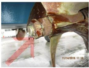
Damage sighted: Minor damage on 1 blade of port side prop.
