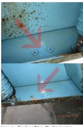
**Hull mounted:** Ground/anode securely mounted on transom. Good condition. No deterioration
