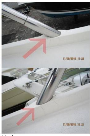
**Toe rail(s):** Molded in, no cracks or separation sighted.
