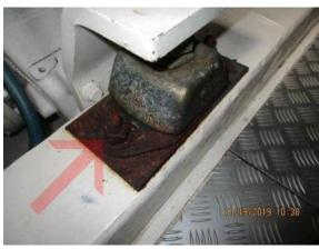
**Drip** pad(s): No Pads in place beneath engine(s). Fluids and debris fall into bilge area. Consider
