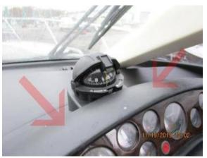
**Compass(es):** Mounted at lower helm and upper helm: 6" Plastimo offshore 105.
